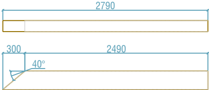
Pilares - Chapa dobrada 250x150 #2.65mm
